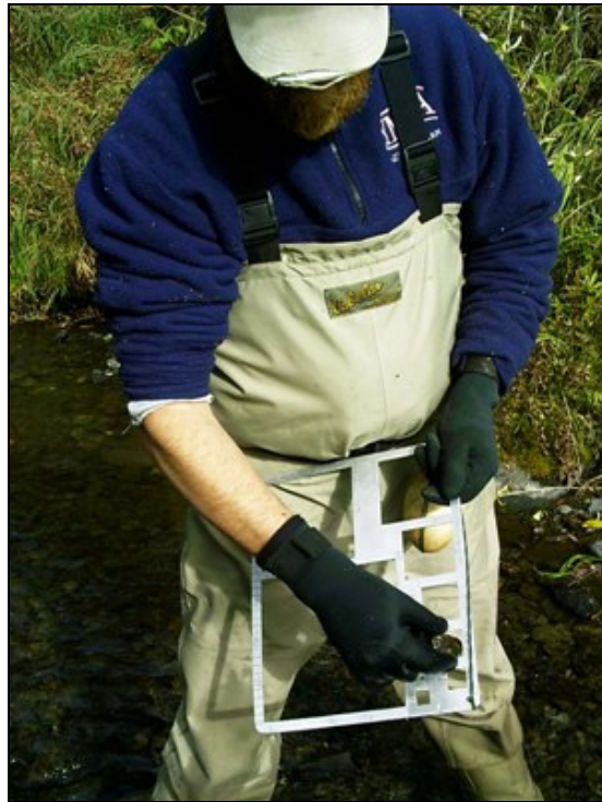
Figure 6. Substrate Sizing Using Wolman Pebble Meter, or “Gravelometer.”
