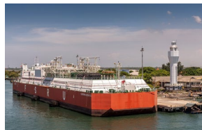
Floating storage plus onboard regasification smaller vessels are barges towed by tugs
