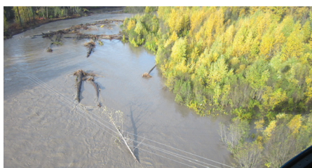
Flooding on the Chuitna River dropped a cottonwood tree into a distribution line, cutting service to Tyonek and Granite Point.
