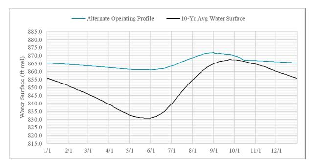
Figure 4-2. Water Surface Elevation Comparison – Existing Dam Releases.
