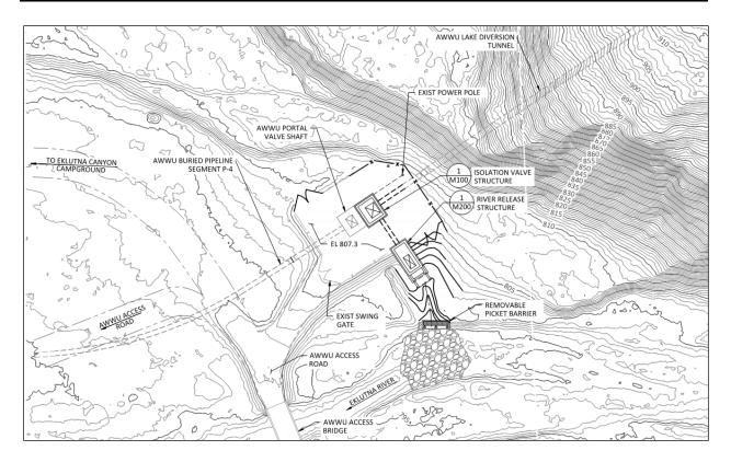
Figure 3-1. Eklutna River Release Facility Site Layout.
